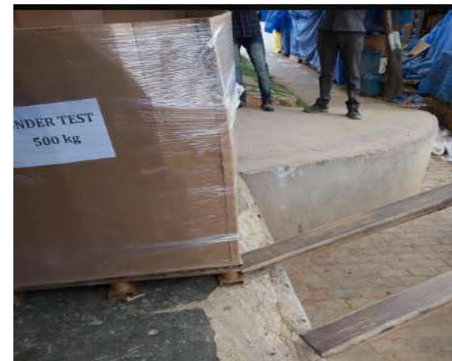
DYNAMIC LOAD TEST OF 500 KGS WITH FORK LIFT PUSHING PALLET CORNER
