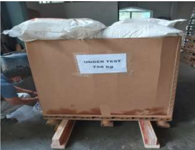
STATIC RACK TEST 750 KGS WITH PALLET WETTING OVER 3 DAYS
