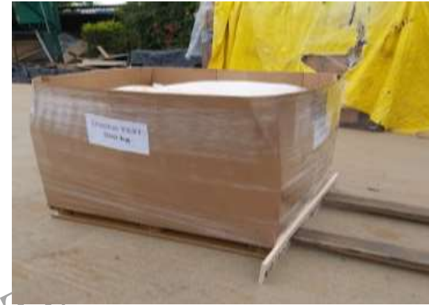
DYNAMIC DRAG TEST ON ROUGH FLOOR WITH 500 KGS
