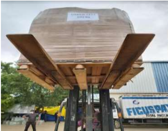
DYNAMIC LOAD TEST OF 500 KGS BY FORK LIFT
